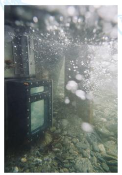
The cameras can be set to record continuously over userdefined intervals, or dynamically using specified motion detection events. When in event detection mode, the user defines a region of the image, which is monitored for motion, after which video is recorded.
