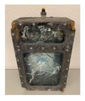
**Example 4**: Camera system (from example 3) after a massive landslide, the camera housing was torn off the rock wall and recovered approximately 2 km below the installation site. The housing and safety glass are massively damaged, but no water penetration into the camera system, which is technically still fully functional and all data on the internal storage was retrieved successfully.
